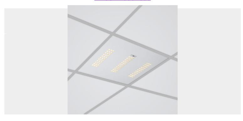
A range of recessed luminaires with medium power LED modules using Multioptic® lens technology, specially designed for use in combination with exposed grid ceilings. Myos-M 600x600 Multioptic contains a set of 99 medium wattage LEDs behind a decorative aperture mask. Each LED is fitted with an individual secondary lens providing superb light distribution. The housing is made of steel, powder coated RAL9016 or RAL9010 with a textured finish.
