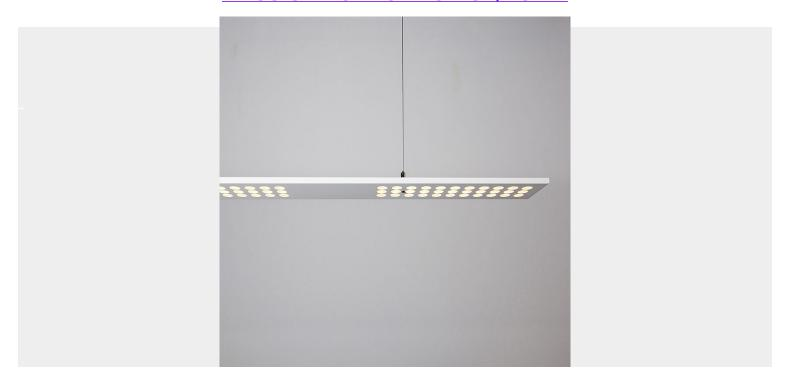
Myos-S2 Multioptic Up/Down is an innovative pendant luminaire with mid power LED-modules using Multioptic® lens technology. Contains 5 modules of 33 power LEDs each behind a decorative aperture mask. Three modules are facing downwards for effective illumination of the working area and two modules are facing upwards providing indirect lighting.
