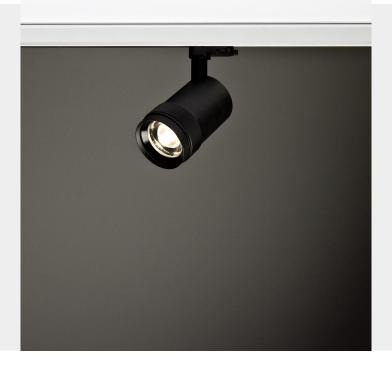
Zumo 90 Vario is a zoomable LED spotlight for standard 3-circuit tracks. The spotlight features a high power LED with a high color rendering index (CRI>97). The light beam can be infinitely adjusted from 12° spot to 55° wide flood by simply turning the zoom lens. Zumo 90 Vario spotlights are particularly suitable for illumination of galleries, museums and art exhibitions.
