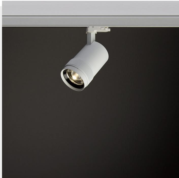
Zumo 90 Vario is a zoomable LED spotlight for standard 3-circuit tracks. The spotlight features a high power LED with a high colour rendering index (CRI>97). The light beam can be infinitely adjusted from 12° spot to 55° wide flood by simply turning the zoom lens. Zumo 90 Vario spotlights are particularly suitable for illumination of galleries, museums and art exhibitions.
