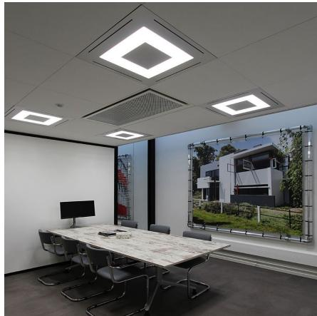
Fusion-CG, a range of LED luminaires with modular dimensions for use in suspended ceilings with concealed grid structures. The luminaires are made of a lightweight composite panel material consisting of two layers of painted aluminum skin with a thermoplastic core in between. The material has excellent thermal and fire resistance values, sound insulation and is extremely flat.
