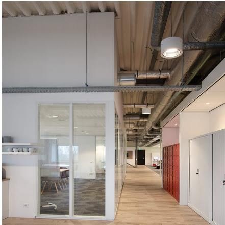
Meson Pro 190-S is a series of suspended LED downlights equipped with a glare-reducing reflector and satin diffuser. The innovative design of LED array, light chamber, reflector and diffuser forms an optical system with high system efficiency and excellent visual comfort. Meson Pro 190-S has a highly effective Light Output Ratio (LOR) of better than 84% and a Unified Glare Rating (UGR) between 16 and 19, depending on the fixture output.
