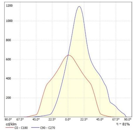
Meson round 190 wallwasher is a high-quality LED recessed downlight with asymmetric light distribution. To ensure uniform lighting across the entire surface, the distance to the wall for wallwashers must not exceed 50-60 cm. The central unit can be rotated within the trim ring to adjust the beam direction.
