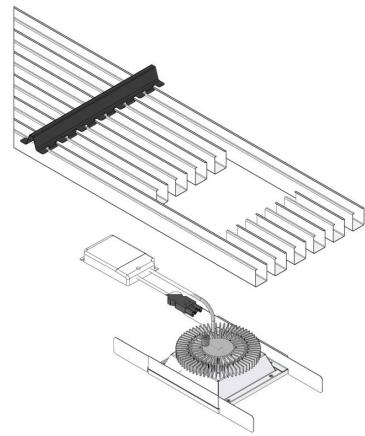
Meson square 180 cardanic SAPP is a series of LED recessed spotlights suitable for use in Interalu SAPP® ceilings. A cardanic mechanism allows easy adjustment of the spot up to 30° in all directions.
