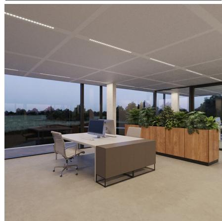
Metronome-K is a linear LED luminaire equipped with 20, 28, or 36 lenses, recessed behind a grid louver. This LED luminaire offers a completely new lighting solution for effective illumination with an architectural aesthetic. A choice can be made between UGR< 19 optics (standard) and UGR< 16.
