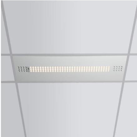
Myos-M Multioptic Linear is a series of innovative recessed luminaires with mid-power LED modules, utilizing Multioptic® lens technology, specifically designed for use with visible grid suspended ceilings. The optical system features a lens array of 99 mid-power LEDs behind a decorative diaphragm mask.
