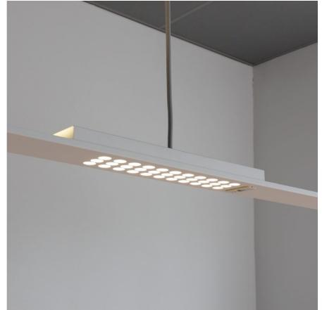
Myos-S2 Multioptic Up/Down is an innovative pendant luminaire with mid-power LED modules that use Multioptic® lens technology. It contains 5 modules of 33 power LEDs each behind a decorative diaphragm mask. Three modules are directed downwards for effective illumination of the work area and two modules are directed upwards for indirect lighting.
