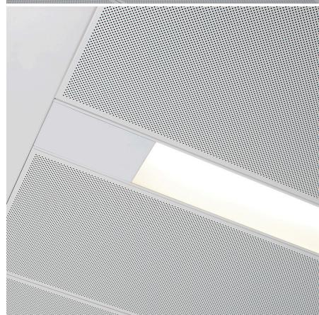
Stratos-K 100 is a linear LED luminaire designed for use in climate ceilings with visible grid systems. The luminaire is shielded by a microprismatic lens (with a UGR<19 for office applications according to NEN-EN 12.464/1).
