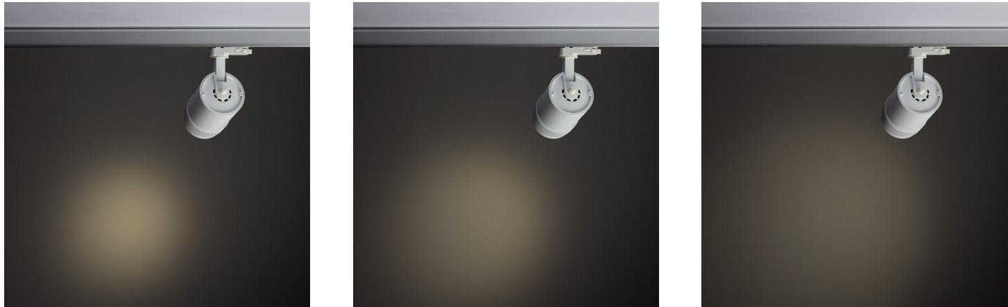
Zumo 100 Vario is a zoomable LED spotlight for standard track rails. The spotlight features a powerful LED with a high color rendering index (CRI> 97). The light beam can be continuously adjusted from 12° spot to 55° wide flood by simply rotating the zoom lens. Zumo 100 Vario spotlights are particularly suitable for lighting galleries, museums and art exhibitions.
