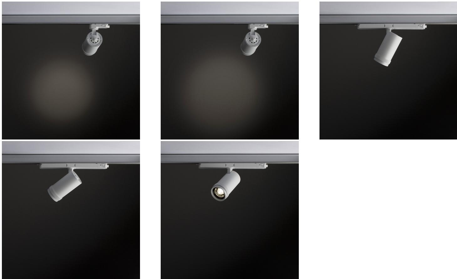
Zumo 60 Vario is a zoomable LED spotlight for standard 3-phase track systems. The spotlight features a powerful LED with a high color rendering index (CRI > 97). The light beam can be continuously adjusted from 10° spot to 50° wide flood by simply rotating the zoom lens. Zumo 60 Vario spotlights are particularly suitable for lighting galleries, museums and art exhibitions.
