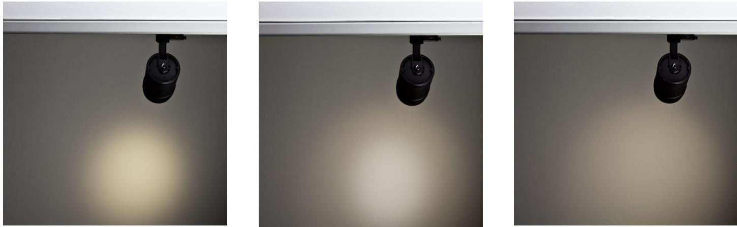
Zumo 90 Vario is a zoomable LED spotlight for standard 3-phase tracks. The spot features a powerful LED with a high color rendering index (CRI> 97). The light beam can be continuously adjusted from 12° spot to 55° wide flood by simply rotating the zoom lens. Zumo 90 Vario spotlights are particularly suitable for illuminating galleries, museums, and art exhibitions.
