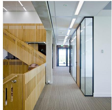
Fusion-BM is a modular LED luminaire crafted from steel for specific application in exposed grid ceilings. The insert modules are developed as an alternative to T8 and T5 fluorescent luminaires for renovation and new construction projects. Fusion-BM is equipped with micoprismatic lens optics featuring low surface luminance (UGR < 19).
