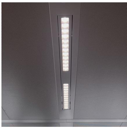
Metronome 12+12 is a linear LED luminaire equipped with two rows of 12 lenses, decoratively recessed behind a grid-like louver. The luminaire features magnetic mounting, making installation easy in ceilings with existing cutouts. The lens and louver design results in an innovative lighting solution for effective illumination with an architectural aesthetic. There is an option to choose between UGR< 19 optics (standard) and UGR< 16 optics.
