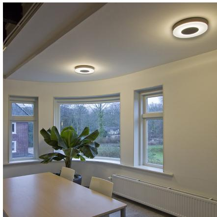
Moonglow round 290 is a surface-mounted fixture with a decorative luminous disc-shaped acrylic diffuser.
