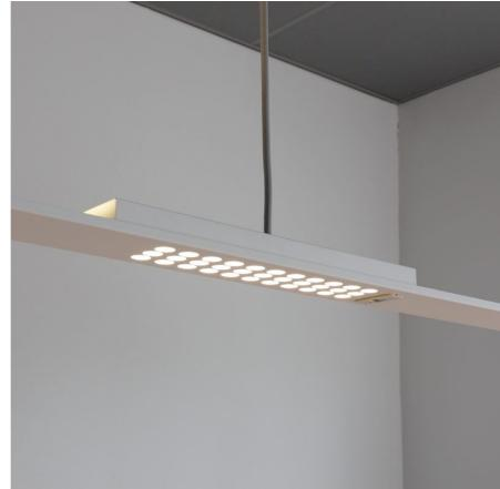
Myos-S2 Multioptic Up/Down is an innovative pendant luminaire with mid-power LED modules that use Multioptic® lens technology. It contains 5 modules of 33 power LEDs each behind a decorative diaphragm mask. Three modules are directed downwards for effective illumination of the work area and two modules are directed upwards for indirect lighting.
