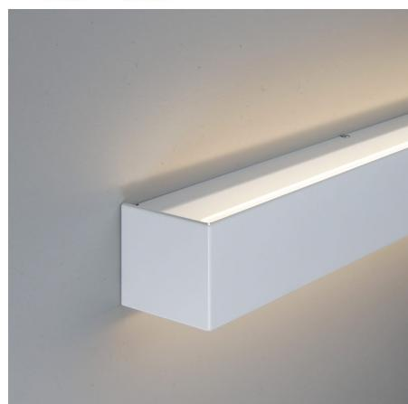
Zender, a wall-mounted LED fixture, is designed for architectural indoor lighting of vertical surfaces such as walls, corridors and stairs. Light emitted by an internally mounted LED strip directed toward the wall is first diffused by a double frosted diffuser and then reflected upward and downward, creating a softly illuminated wall.
